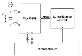
(1): MODE/SPEED config settings (2): DATA/CLOCK outputs
